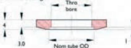
Figure 5 Socket weld
