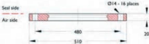
Figure 3 Centring ring assembly
