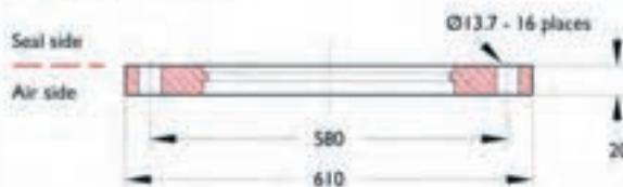
**Figure 3** Centring ring assembly
