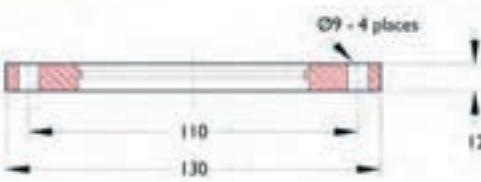
Figure 3 Centring ring assembly
