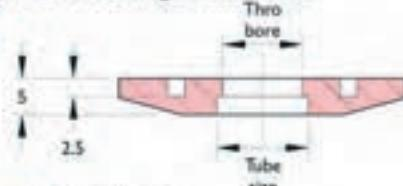
**Figure 4** Weld flange
