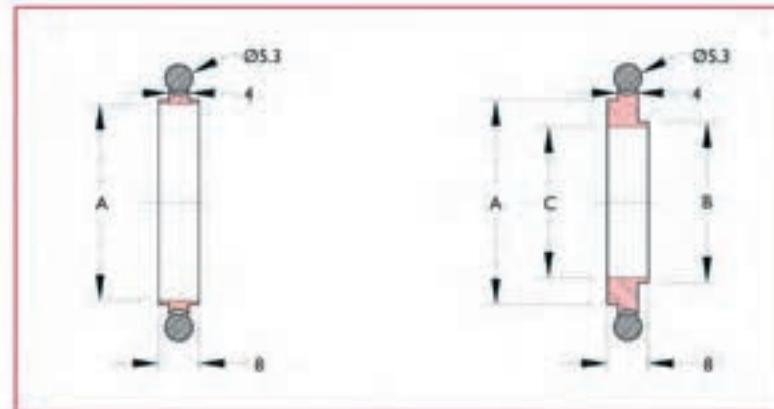
Centring ring assemblies are placed between two ISO flanges with matching outer diameters. The widest portion of the centring ring rests inside a capture groove on the flange and the O-ring rests on the flat polished surface outside the capture groove. On a blank flange, the groove seen on the face of a flange is the capture groove, with the O-ring making contact with this flange face just outside the groove.
