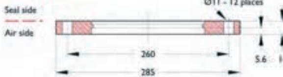
**Figure 3** Centring ring assembly
