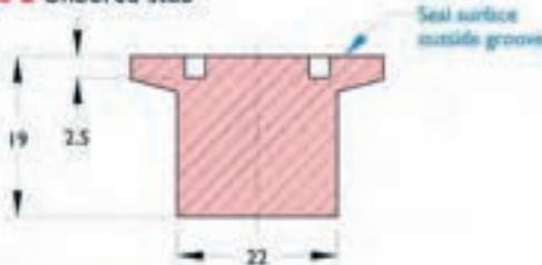
Figure 3 Weld flange – small tube
