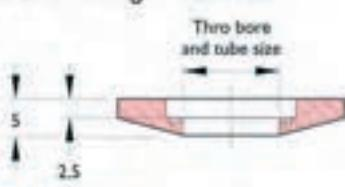
Figure 4 Weld flange
