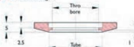
**Figure 5** Socket weld
