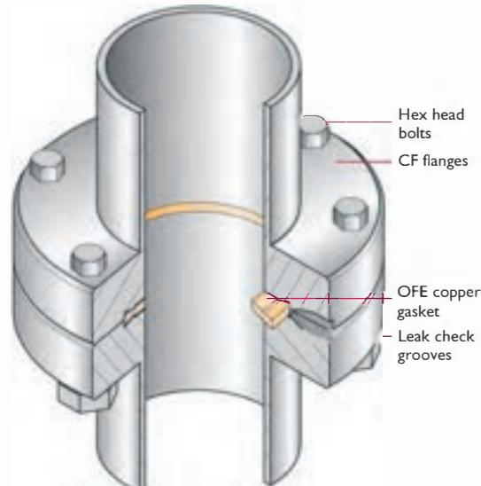
Intermediate hardware may be required for joining components, these have been omitted for clarity
