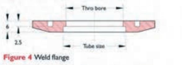
**Figure 4** Weld flange
