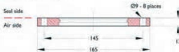
**Figure 3** Centring ring assembly
