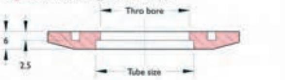
**Figure 4** Weld flange
