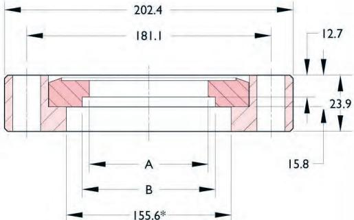
■ Through hole flanges have 20 bolt holes drilled 8.4 diameter
