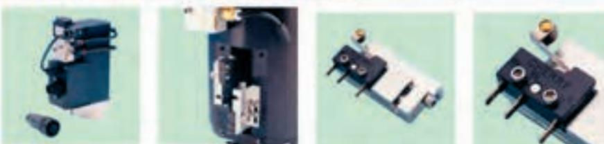
Circular C-Loc™ gate valves can be fitted with optional high precision, modular mechanical position indicators (MPI). This new MPI system consists of two single pole double throw micro switches fitted with integral hinged lever and roller actuators. Each micro switch is wired in a normally open position. Normally closed switches are available on request, and easily modified by reversing standard
