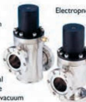
Electropneumatic angle valves with 6.4 to 38mm diameter ports are fitted with air-open/spring-close actuators. Valves with 50mm or larger diameter ports employ air-open/air-close pneumatic actuators. Custom actuator designs are available on request. The solenoid valve temperature should not exceed 50°C. Pneumatically actuated air cylinder seals are FKM / FPM fluoroelastomer O-rings and therefore have a temperature limit of 150°C.
