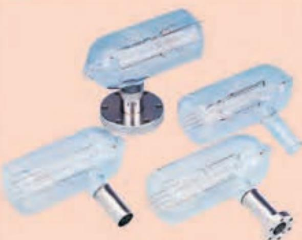
Side arm glass envelope ionization gauge tubes
